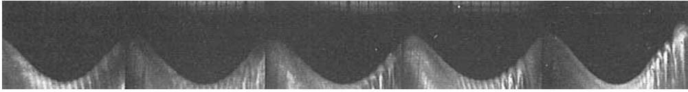
FIGURE 9. An 'extended' spatial series of the 5.26 Hz experiments showing 5 wavelengths of the wave field beginning 0.5 wavelengths downstream of the wave maker.
